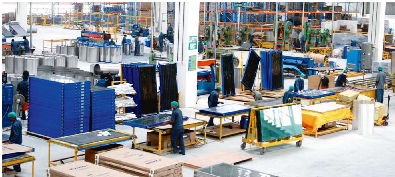
Flat plate collector manufacture in India. The Emmvee production plant opened in summer this year.
